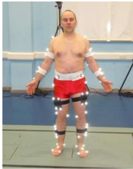
Figure 4.4 Passive retro-reflective markers applied to participant in Calibrated Anatomical Systems Technique (CAST) (Cappozzo et al., 1995)
