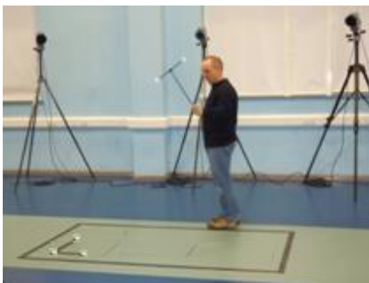
Figure 4.1 Laboratory co-ordinate system and calibration of the image space
