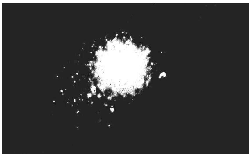
Figure 4. 20: Spray pattern of formulation A2 at 3cm distance from the insufflator device tip (n= 4).
