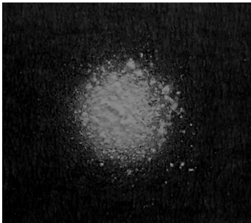
Figure 3. 22: Spray pattern of RH-chitosan microparticles (90:10 w/w, chitosan glutamate to RH) at 3cm distance from the nasal device tip (n= 4).
