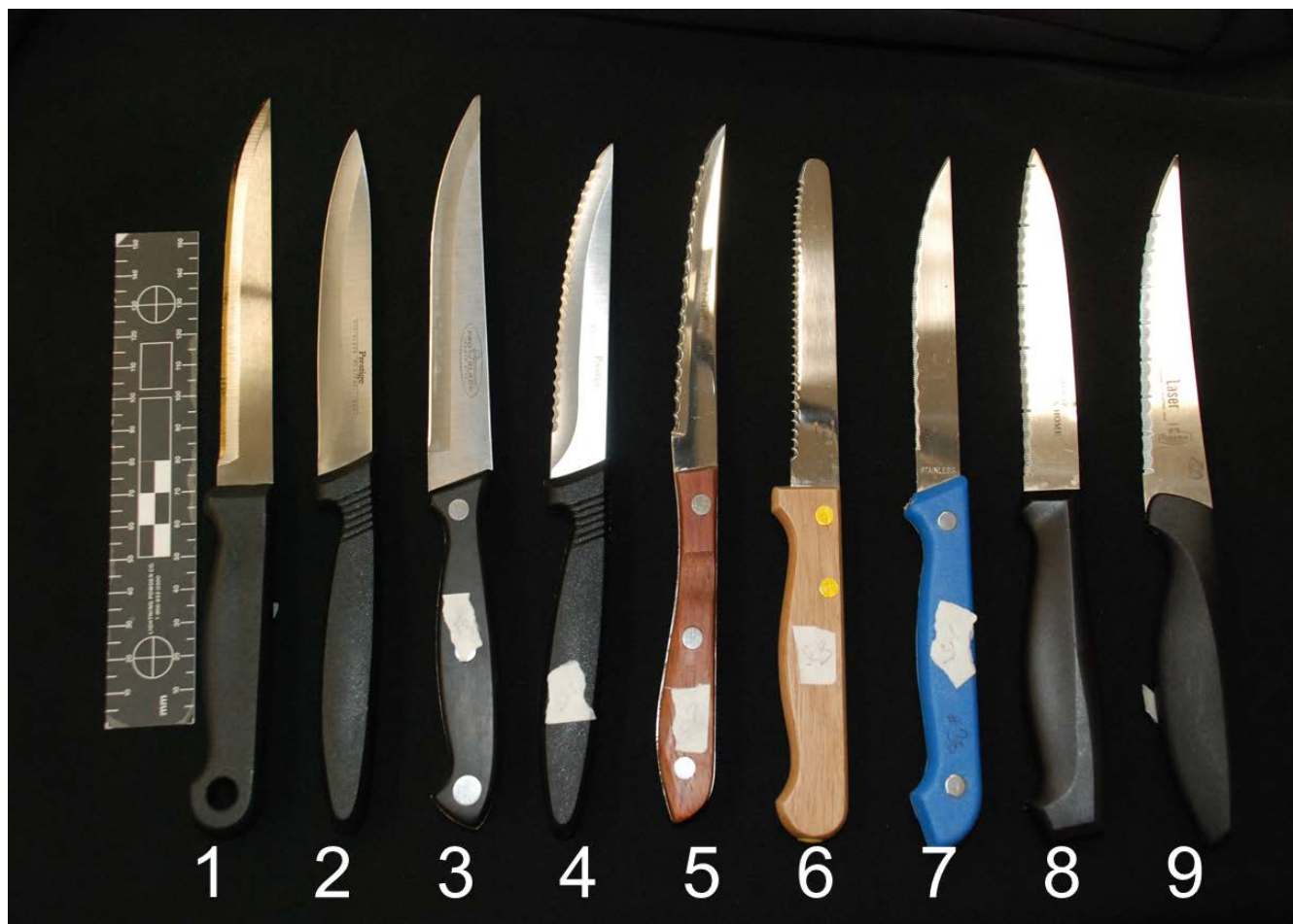
Figure 5.2: Knife sample set of utility blades. 1-3 are fine-edged, 4-6 are scalloped-edged, and 7-9 are serrated-edged blades.
