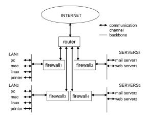
Figure 7. Default network topology adapted from Suehring [22]
