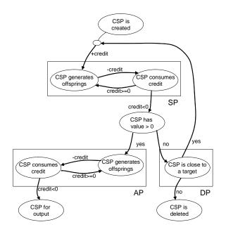
Figure 1. Life-cycle of a CSP
