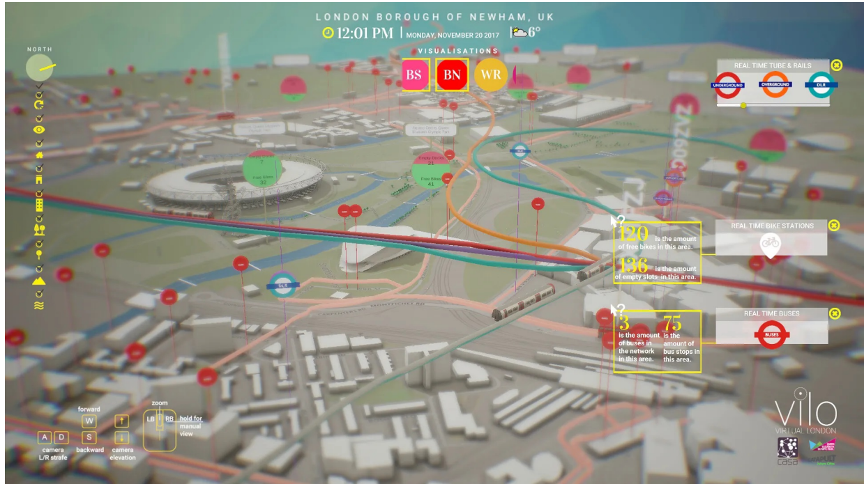
Figure A.7. Simulation of reality through DTs: ViLO model showing live sensor data on infrastructure equipped with VR and AR [74]. A digital model of the Queen Elizabeth Olympic Park in London, UK, is enriched with real-time data streams and connected to the ViLo Digital Platform for Data Visualizations in Participatory Urban Planning. Image courtesy of The Bartlett Centre for Advanced Spatial Analysis ( https://www.ucl.ac.uk/bartlett/casa ).
