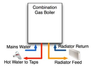
Figure 1. Combination ('Combi') Gas Boiler
