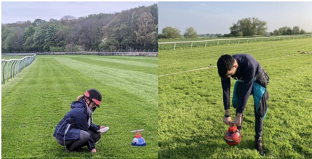
Figure 2.1. The Vienna Surface Tester (instrumented ball) and a ThetaProbe (three-pronged moisture meter used to measure volumetric moisture content) are used to assess surface functional properties.
