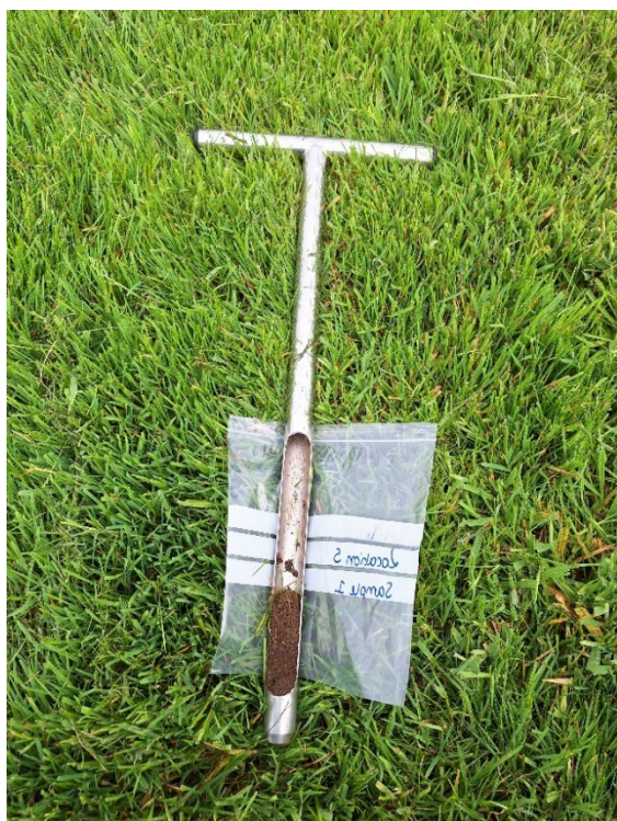
Figure 4.1: Example of soil core taken from seven racecourses out of season to analyse the influence soil texture has on surface functional properties
