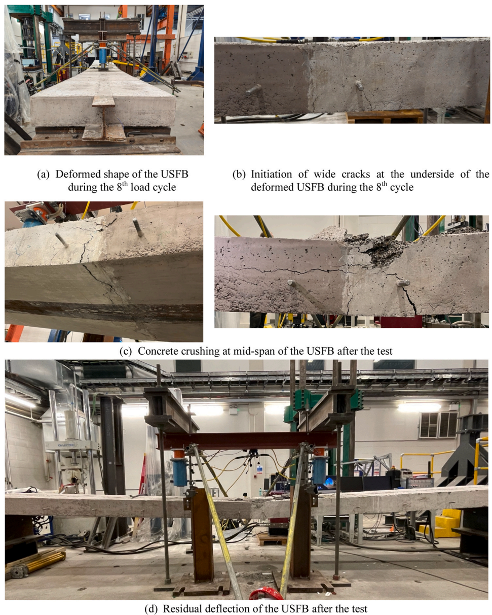
Fig. 10. Failure modes of the composite USFB.
