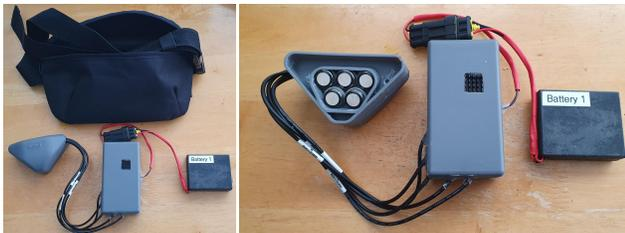
Fig. 3: The advanced MyPAD device: i) US transmitter, ii) US receivers, iii) US electronics, iv) PCB, and v) AI unit.
