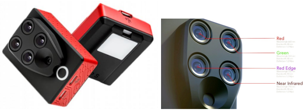
Fig. 5: Multi-spectral RGB camera: Parrot SEQUOIA + multi-spectral sensor.
