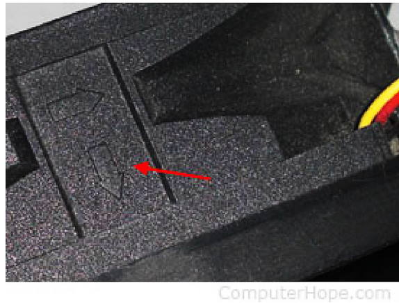
Fig. 6. Signs on ventilator specify fan blades rotation and airflow direction [7].
