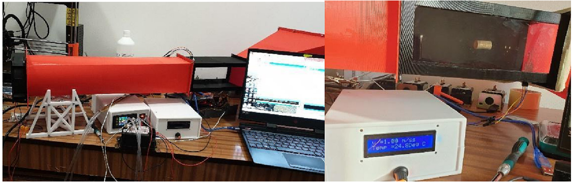
Fig. 16. Assembled wind tunnel during calibration of bi-directional pressure probe.
