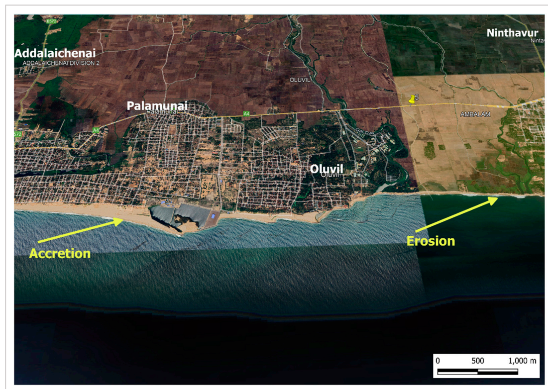
Figure 8. Eroded and accreted areas in the Oluvil coastline (accessed on 7 January 2023).
