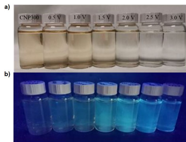
Figure 3. Photos of 0.02 mg ml -1 C-dots dispersions in 0.15 M KCl that has been subjected to chronoamperometry treatments for 60 s at applied voltages from 0.5 to 3.0 V compared to the untreated sample under (a) daylight and (b) UV-radiation.
