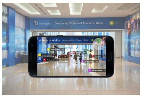
Fig. 2. Concept design for a prototype location-based AR asset management app in an airport for utility managers
