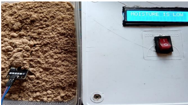
Fig. 5 response of the soil sensor when moisture content is low
