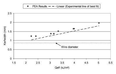
Figure 11. Comparison between FEA and experimental Kerfwidths (XPS, 0.91 mm wire).
