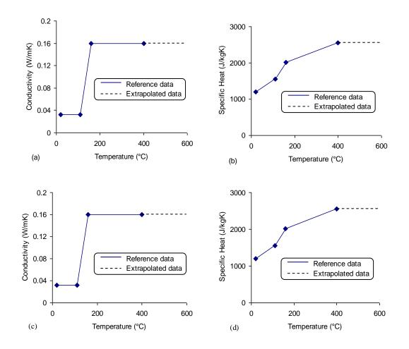
Figure 5. Thermal material properties of PS. a) EPS conductivity b) EPS specific heat c) XPS conductivity d) XPS specific heat.
