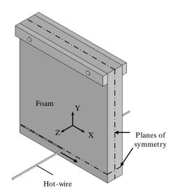
Figure 4. Graphical representation of the hot-wire cutting process.
