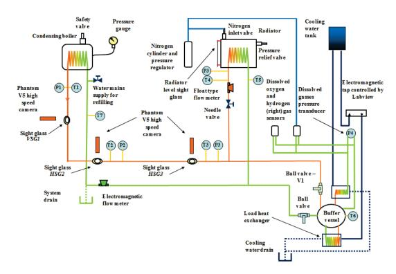
Figure 2: Schematic diagram of experimental set up
