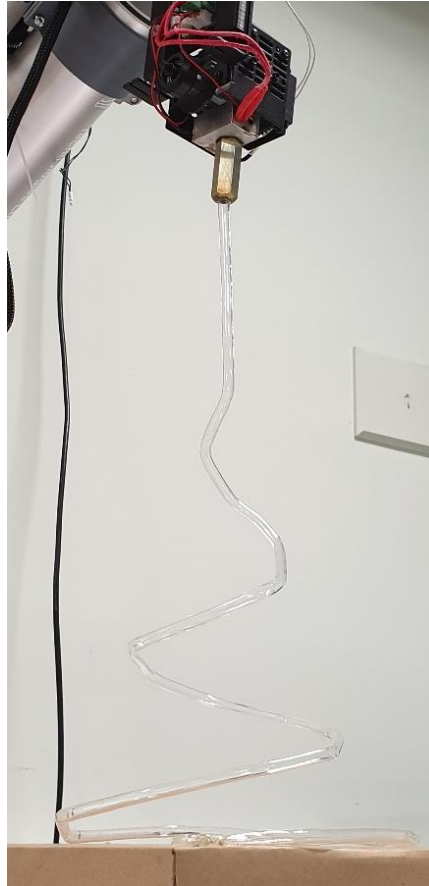
Figure 16. Freeform printing of a self-supporting spiral tube. No internal tube pressurisation required.
