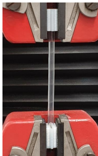
Figure 10. Tube tensile test apparatus with compliant fixtures to prevent tube collapse.
