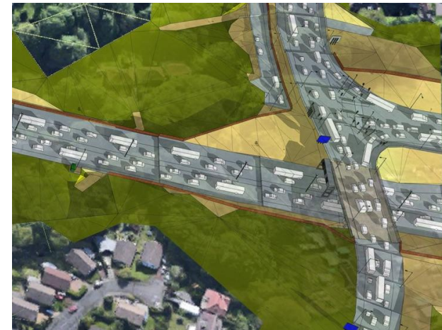
Proposed, detail at Marple Road below Grey = road Light brown = SEMMS topography Dark green = adjusted cut and fill for SEMMS
