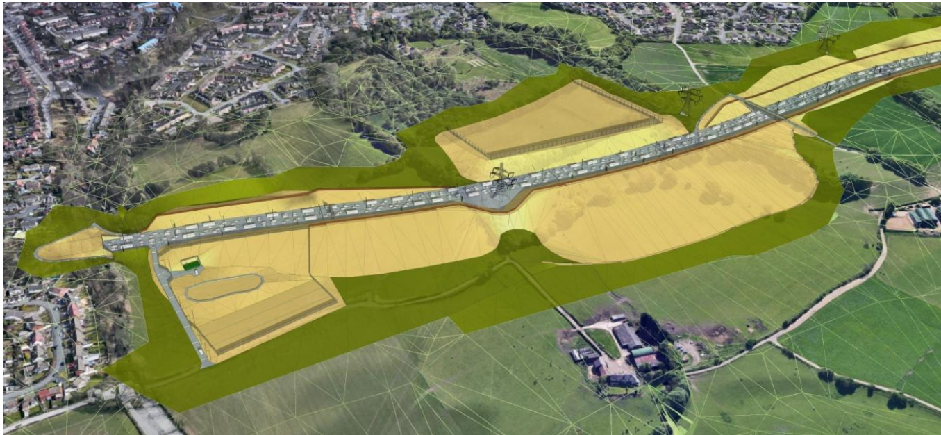
Proposed, detail at lane to Goyt Hall below Grey = road Light brown = SEMMS topography Dark green = adjusted cut and fill for SEMMS
