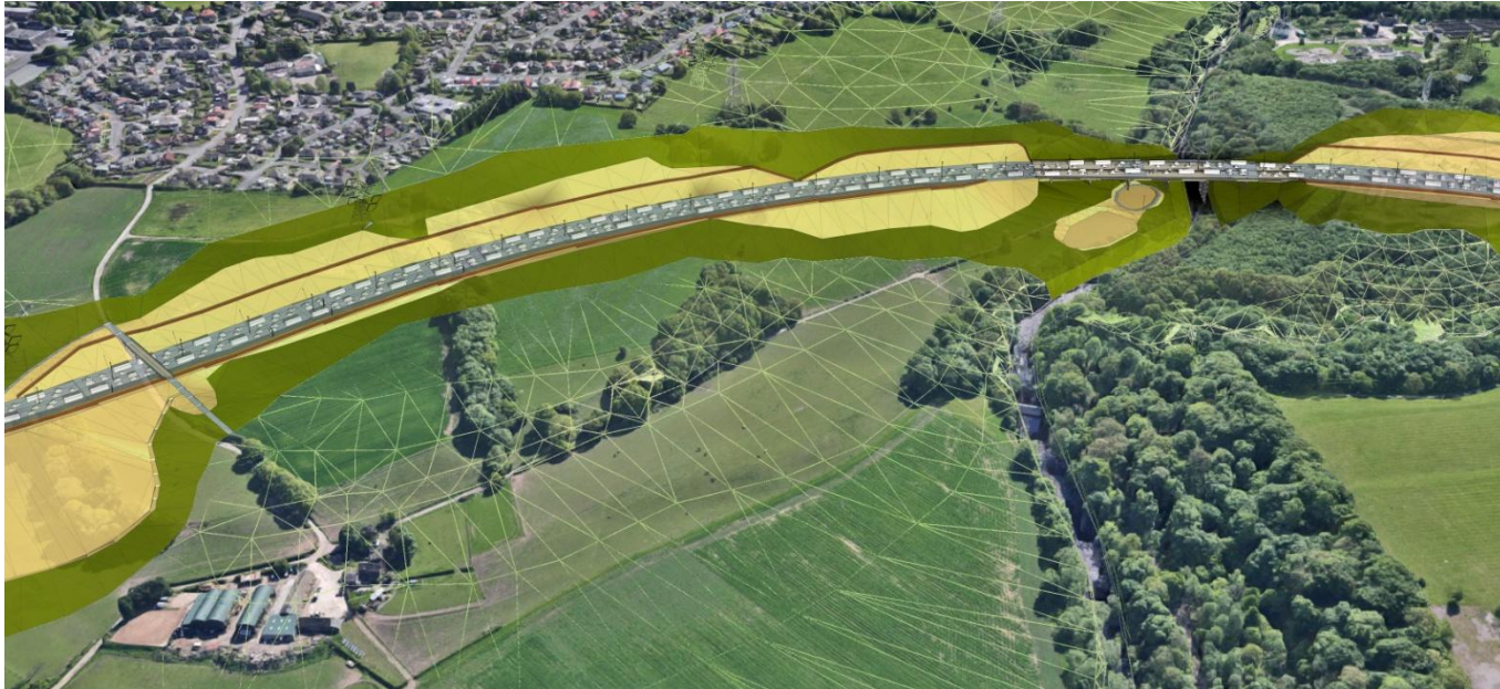
Proposed, detail at Goyt crossing below Grey = road Light brown = SEMMS topography Dark green = adjusted cut and fill for SEMMS
