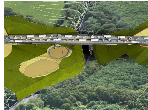
Proposed, detail at Goyt crossing below Grey = road Light brown = SEMMS topography Dark green = adjusted cut and fill for SEMMS
