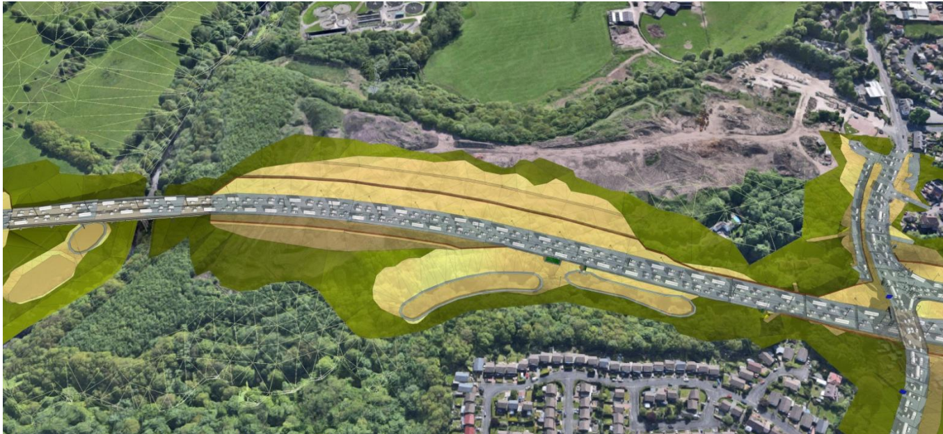
Proposed, detail at Marple Road below Grey = road Light brown = SEMMS topography Dark green = adjusted cut and fill for SEMMS
