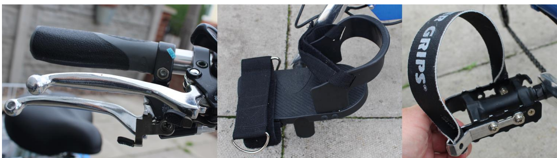
Figure 2: The adaptations available to the stroke survivors. From left to right - repositioned breaks that could be operated simultaneously by the least effected side, a self-levelling pedal with ankle support, and a pedal with a strap attached
