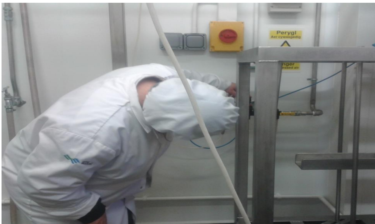
Figure 5. 49 Pressure is being set at 10 psi for 1 hour
