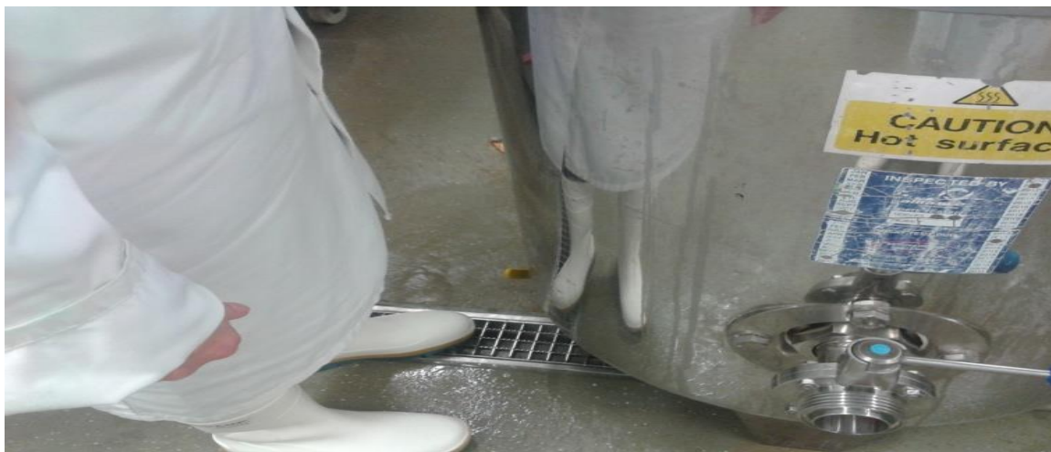
Figure 5. 13 Tap of the pasteuriser from where milk from pasteuriser is transferred into the milk container to be transported into cheese vats
