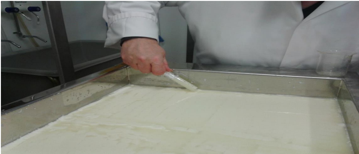
Figure 5. 26 Whey sample extracted using syringe (BD) for testing acidity and pH
