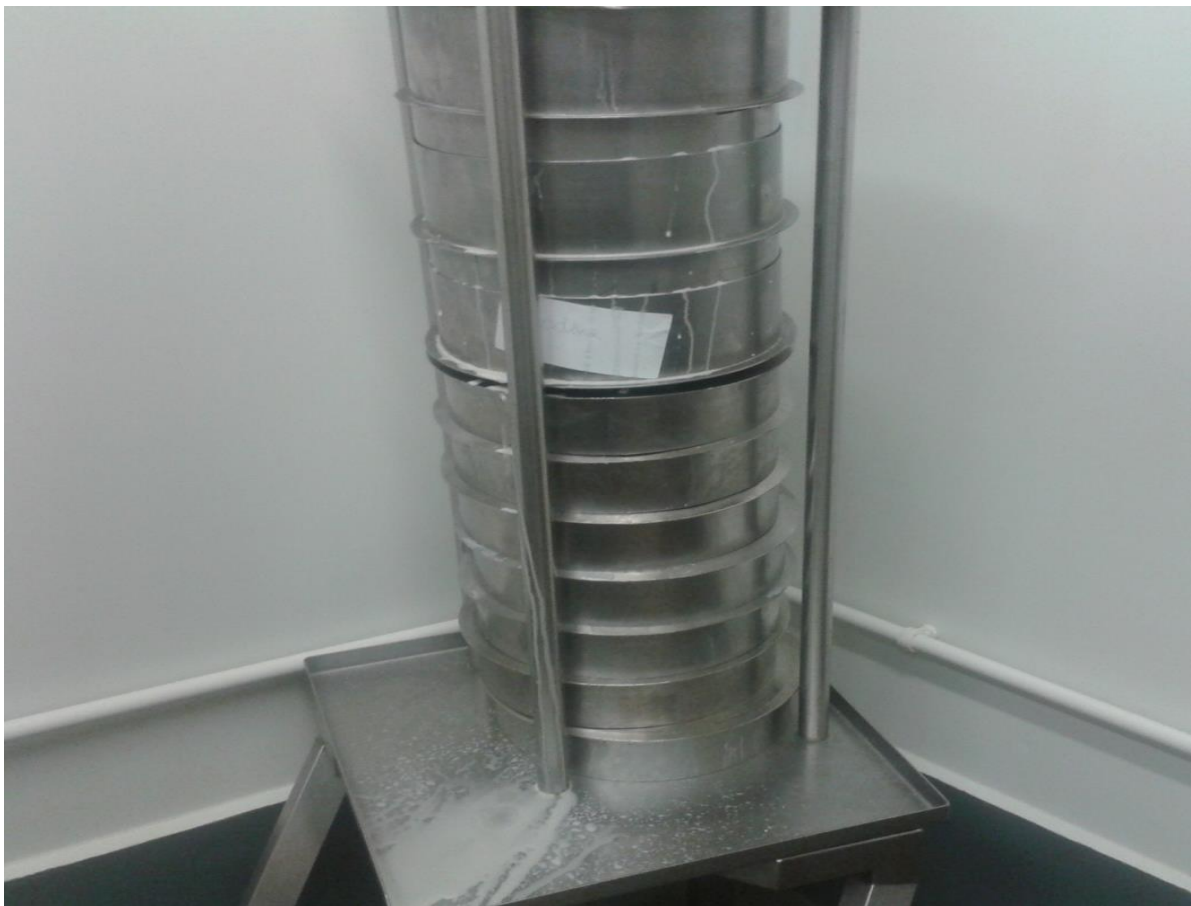
Figure 5. 51 Curd moulds pressed overnight at 80 psi
