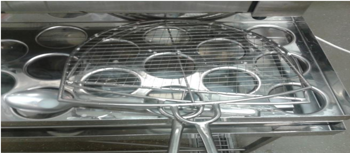
Figure 5. 22 Stainless steel curd cutters
