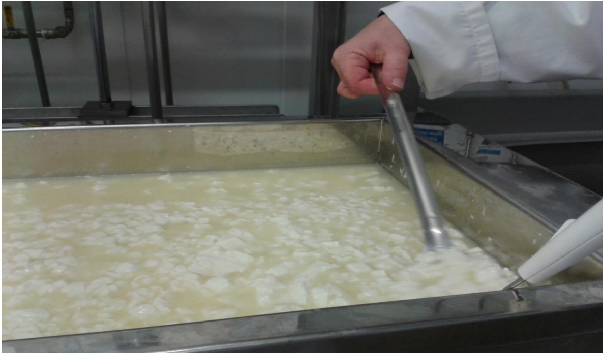
Figure 5. 28 Temperature is checked while stirring at close intervals
