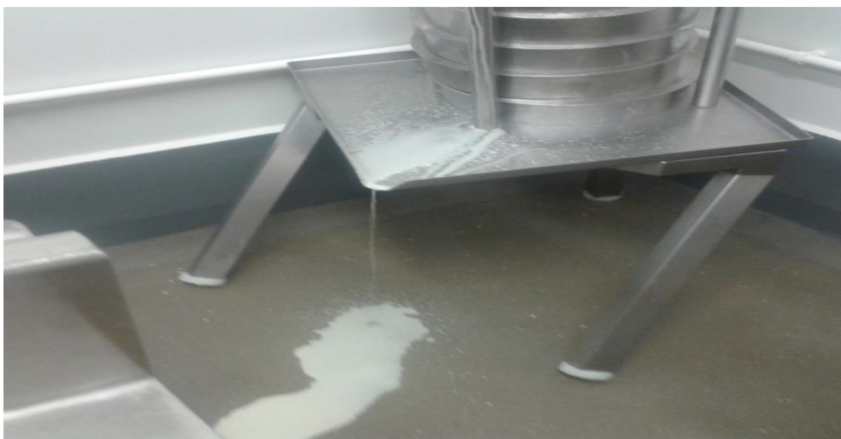
Figure 5. 50 Excess whey released from the moulds upon pressing
