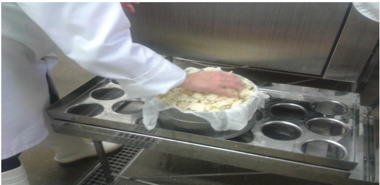
Figure 5. 46 Curd transferred into stainless steel moulds
