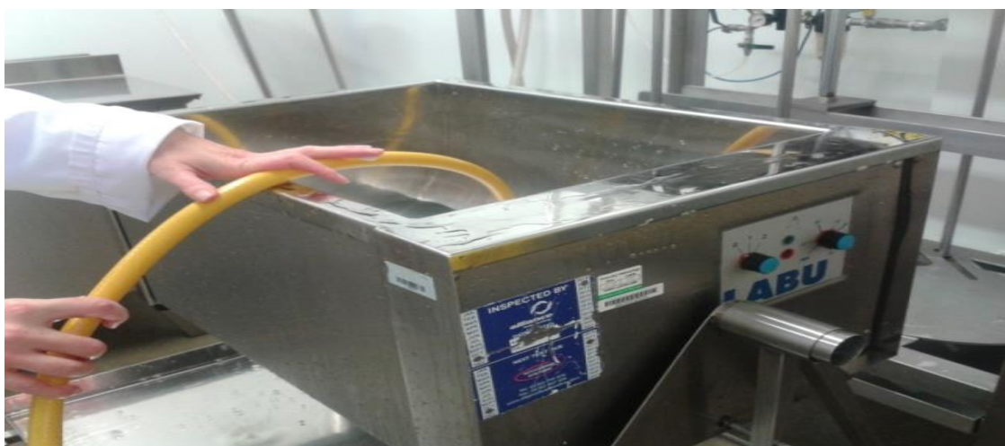
Figure 5. 6 Cheese vat washed using sanitizing solution and thorough cleaning with tap water
