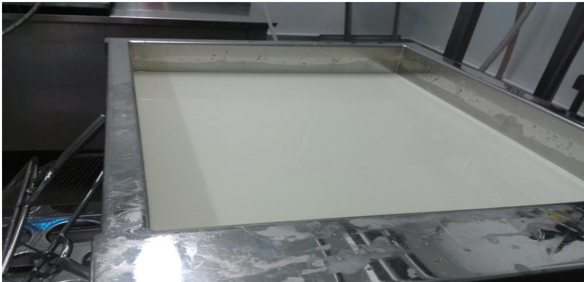
Figure 5. 21 Ripening period of 75 minutes after addition of rennet
