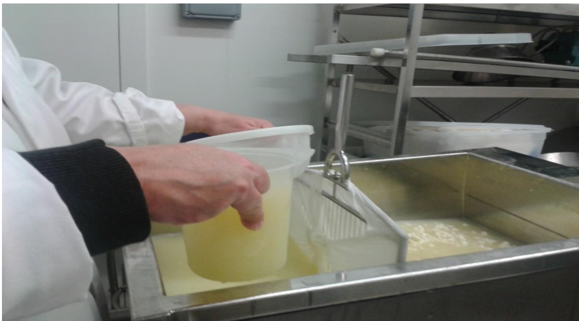
Figure 5. 30 Whey is separated from the curd
