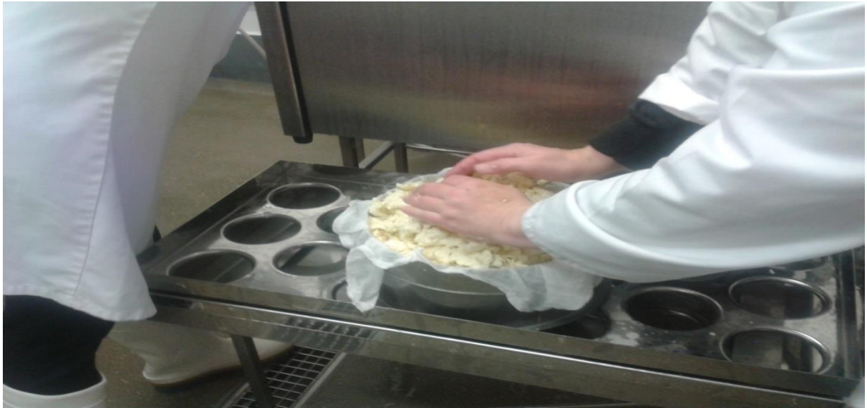
Figure 5. 47 Preparing moulds with curd for pressing in curd pressing machine
