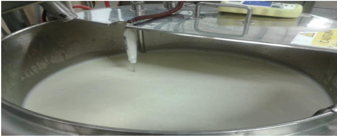
Figure 5. 10 Batch pasteuriser with temperature of the milk being measured
