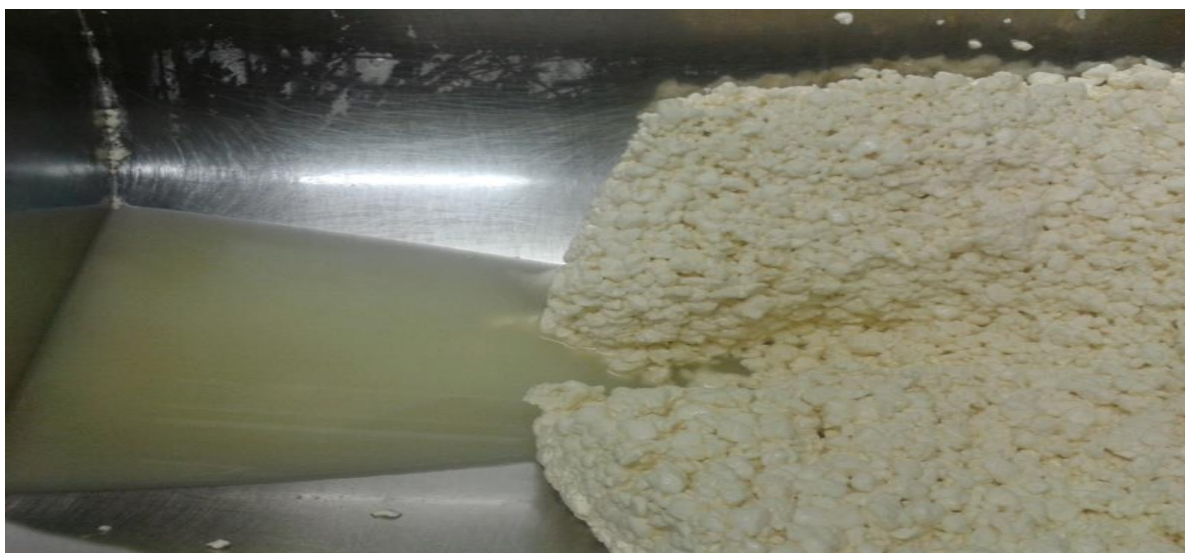
Figure 5. 34 Separating whey from the curd blocks
