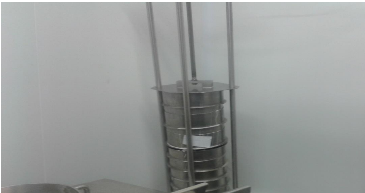
Figure 5. 48 Moulds loaded on the curd pressing machine
