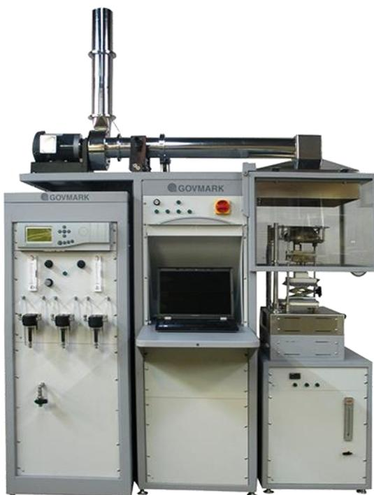
Figure 15 The Govmark CC-2 Cone Calorimeter
