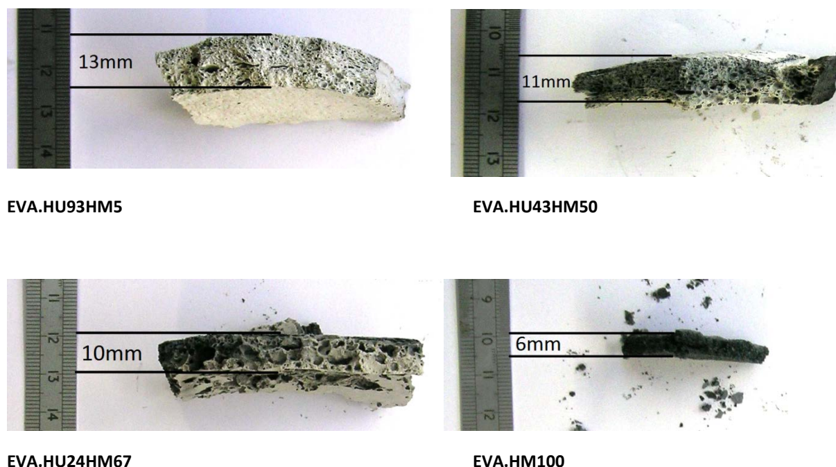
Figure 5: Section through ash of samples containing blends of huntite and hydromagnesite
