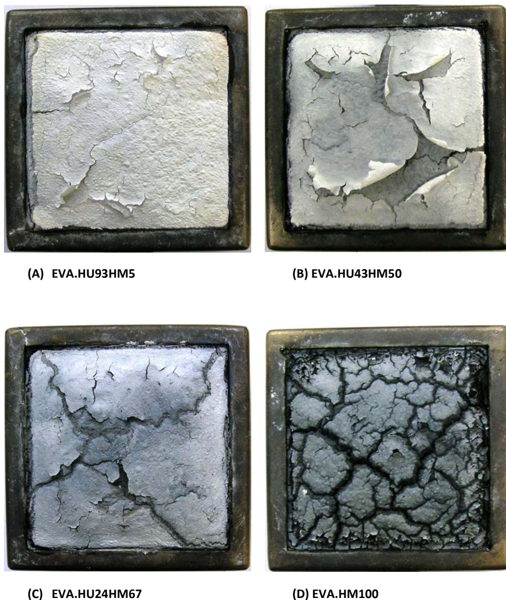
Figure 4: Ash from the cone test of samples containing blends of huntite and hydromagnesite
