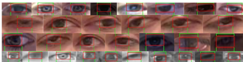
Figure 5. Horizontal and vertical convolution-based pupil coordinates localisation (in randomly selected images from the BIO-ID, GI4E, and Talking-Face datasets) for dynamic conditions such as gaze position, eye colour, intensity, noise interference, eye size, and image resolution.
