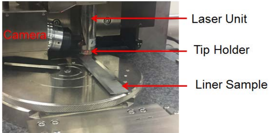
Figure 4: Cylinder Liner Sample undergoing AFM Measurement in Dry Conditions
