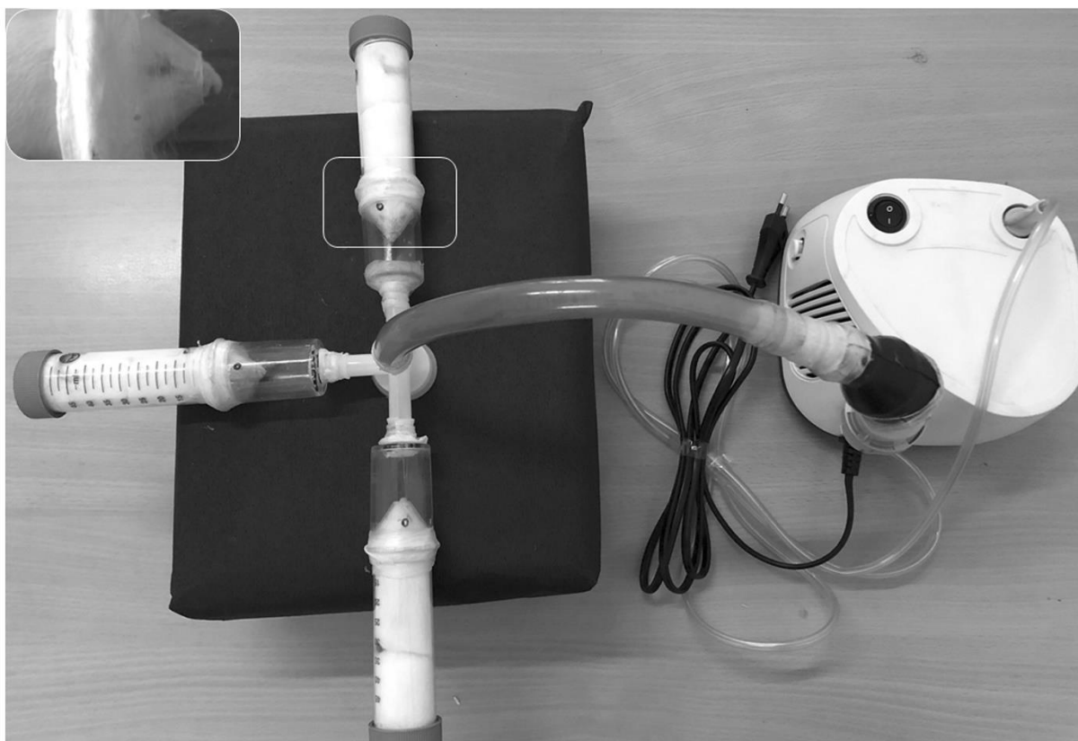
Fig. 3. Design of the inhalation chamber coupled with a nebulizer.
