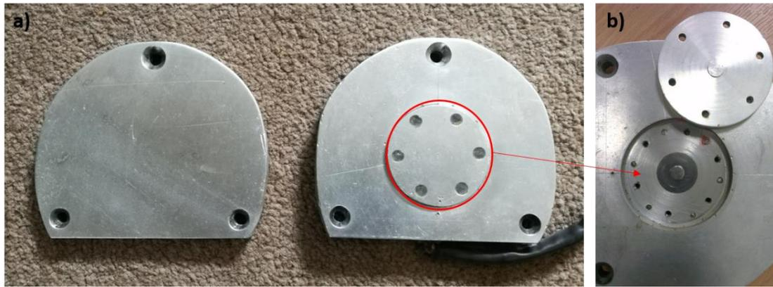
Plate 7.1.3 a: 'Dummy' force shoe (left) and prototype force shoe (right); b: The single axis button load cell (Interface LBS miniature compression load) secured beneath the plate.
