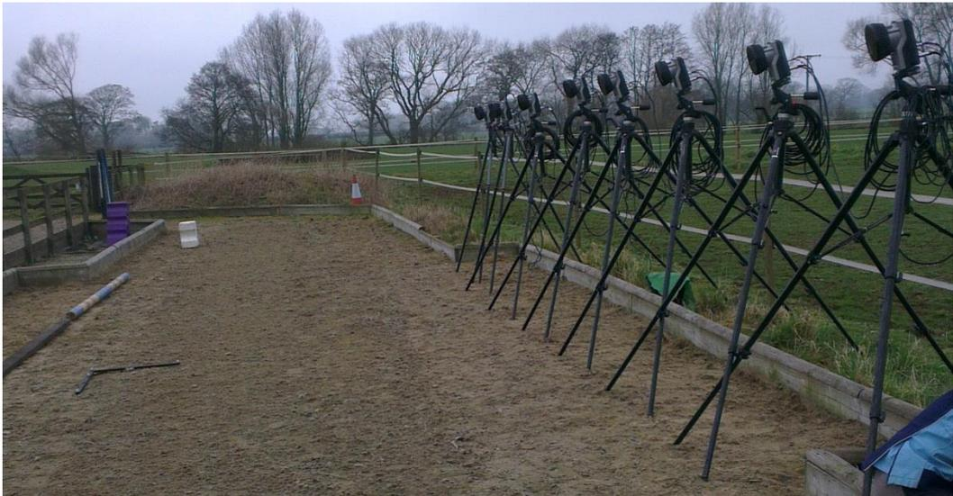
*Plate 4.2.1: An eight camera motion capture system set up for an extended calibration.*
