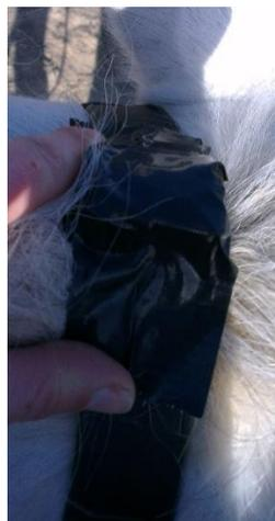
Plate 5.2.6: Accelerometer being secured to the poll of Horse 7.
