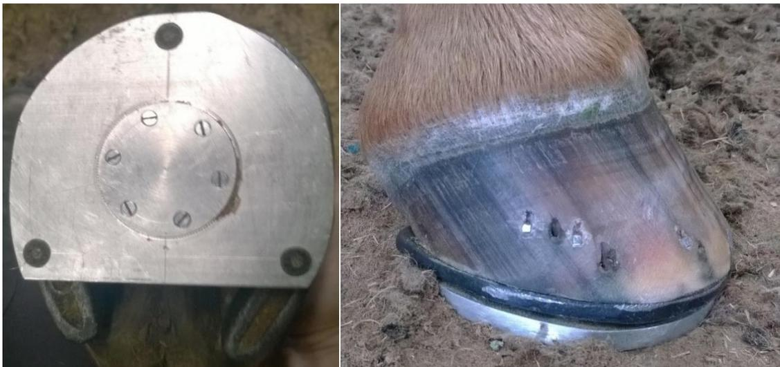
Plate 4a: Solar view of the prototype force shoe secured to the base of the right front shoe.
