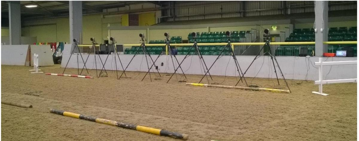
Plate 6: An 8 camera motion analysis system set up for an extended calibration
