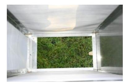
Figure 2 - View from above modified Gerking box sampler with cutting blade retracted to show size of sample obtainable.
