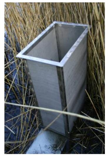
Figure 3- Modified Gerking box sampler within reed bed.
