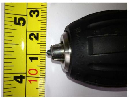
Figure 6.1: A 2mm diameter drill bit was reduced in length and set so that only 2mm protruded from the chuck.
