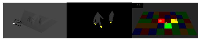
Figure 3: Left: Depth map rendered. Center: Feedback detection with grouping points of interest near the floor surface. Right: Player feet positions projected onto interactive surface.
