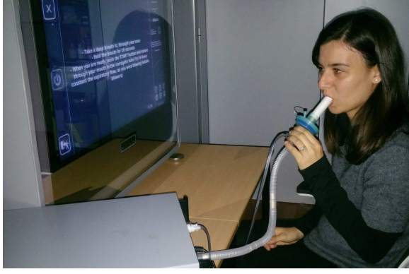
Fig. 13. The Wize Sniffer final configuration. The user blows into the corrugated tube while attempting to keep the expiratory flow rate constant. The flowmeter can be used to calculate the exhaled breath volume. A flushing pump purges the chamber to recover the sensor's steady state between two consecutive measures. The Wize Sniffer was designed to be integrated into the Wize Mirror or to be used as a stand-alone device.
