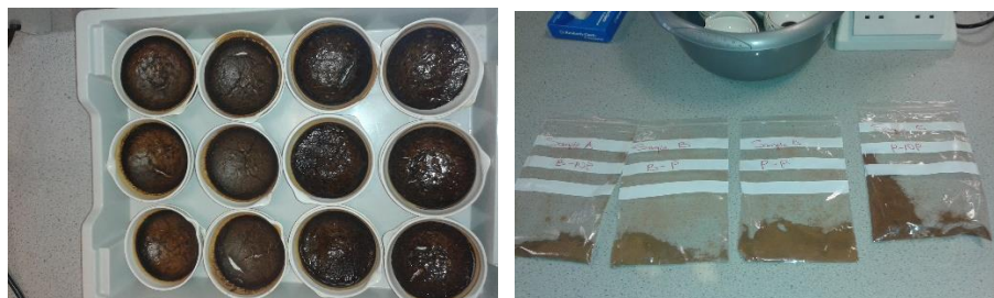
Step 1: Yogurt after drying at 105°C for 16 hours.
