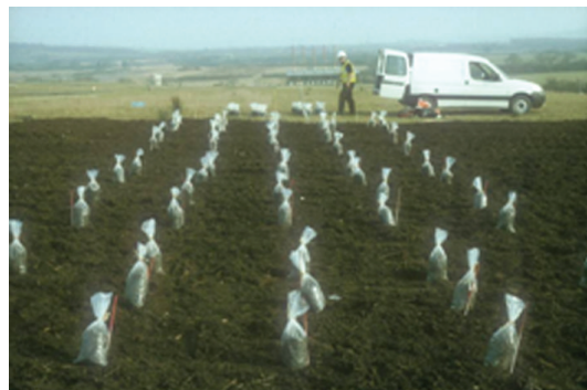
FIGURE 12: Two litre Earthworm Inoculation Units (EIUs) ready for inoculation into an organically-enriched landfill cap in the south of England.
