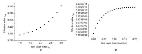
**Fig. 2** Effective index for a three layer waveguide with  $l=1~\mu m$  and  $\Delta \mu=0.23$
