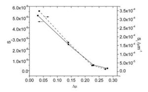
**Fig. 3** Sensitivity of a three-layer waveguide sensor with l=1  $\mu m$  against refractive index step  $\Delta \mu$
