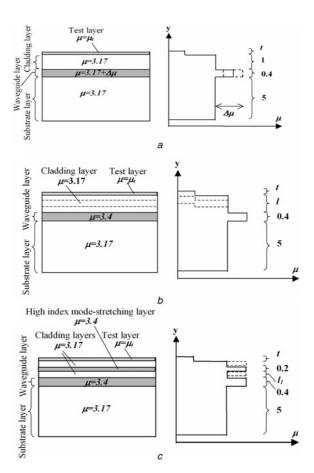
**Fig. 1** Cross sections and refractive index profiles of waveguides investigated (all lengths in  $\mu m$ )
