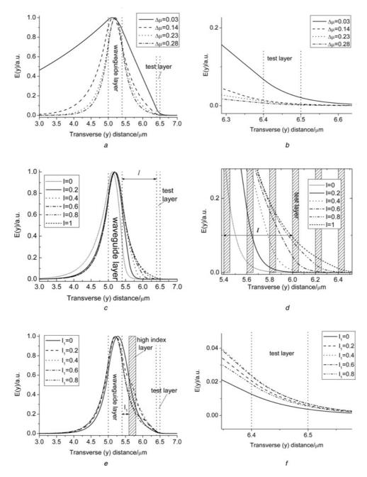
Fig. 6 Mode profiles for the fundamental TE mode in the waveguide structures investigated
