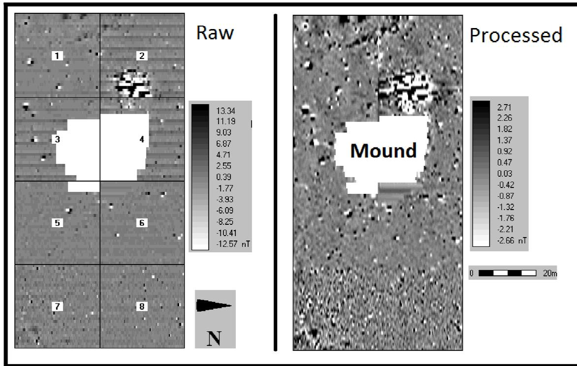
Figure 5.20 Raw and processed gradiometer survey, Area 1 survey 1
