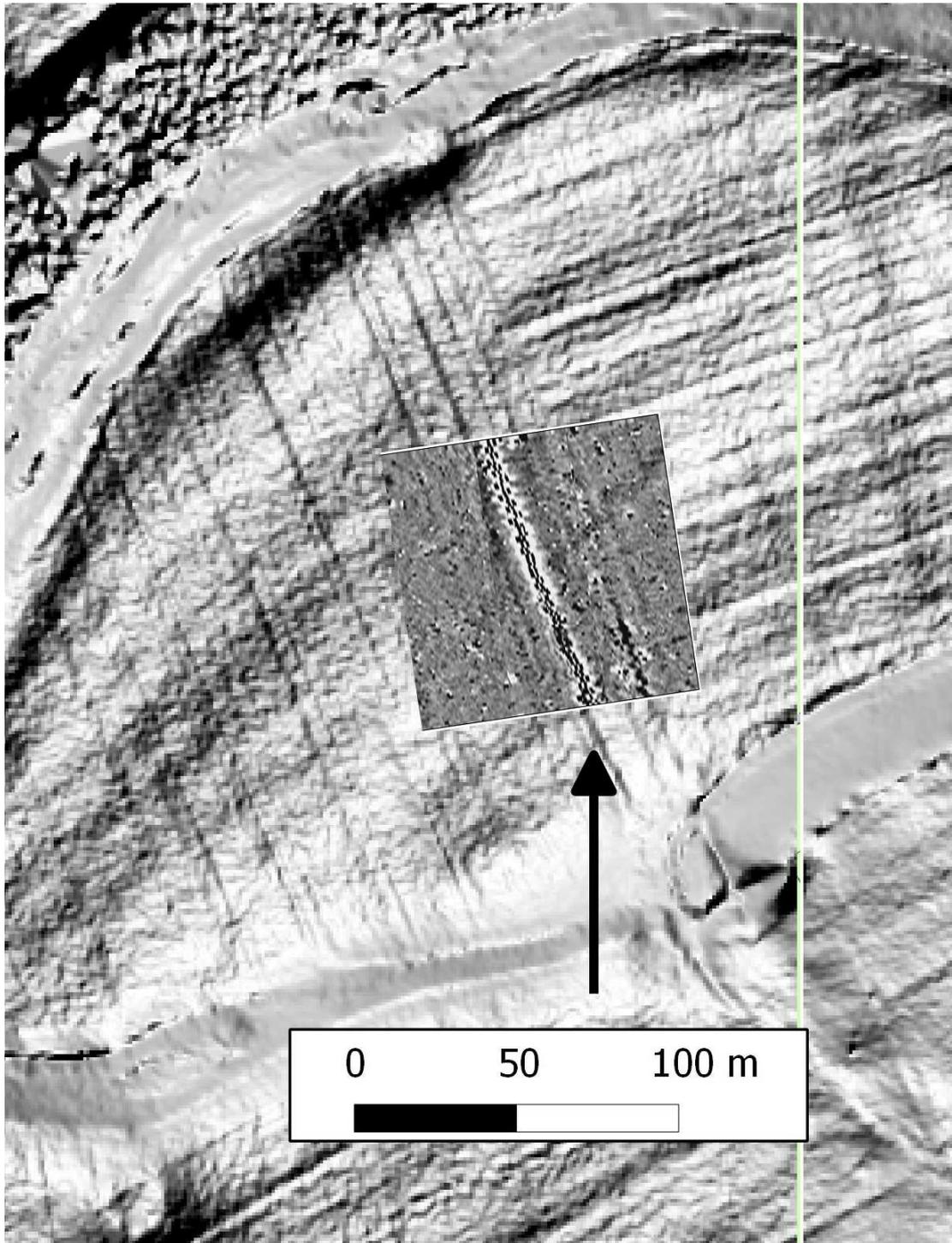
Figure 5.7 Gradiometer survey overlaid onto the LiDAR model of Brockhall
