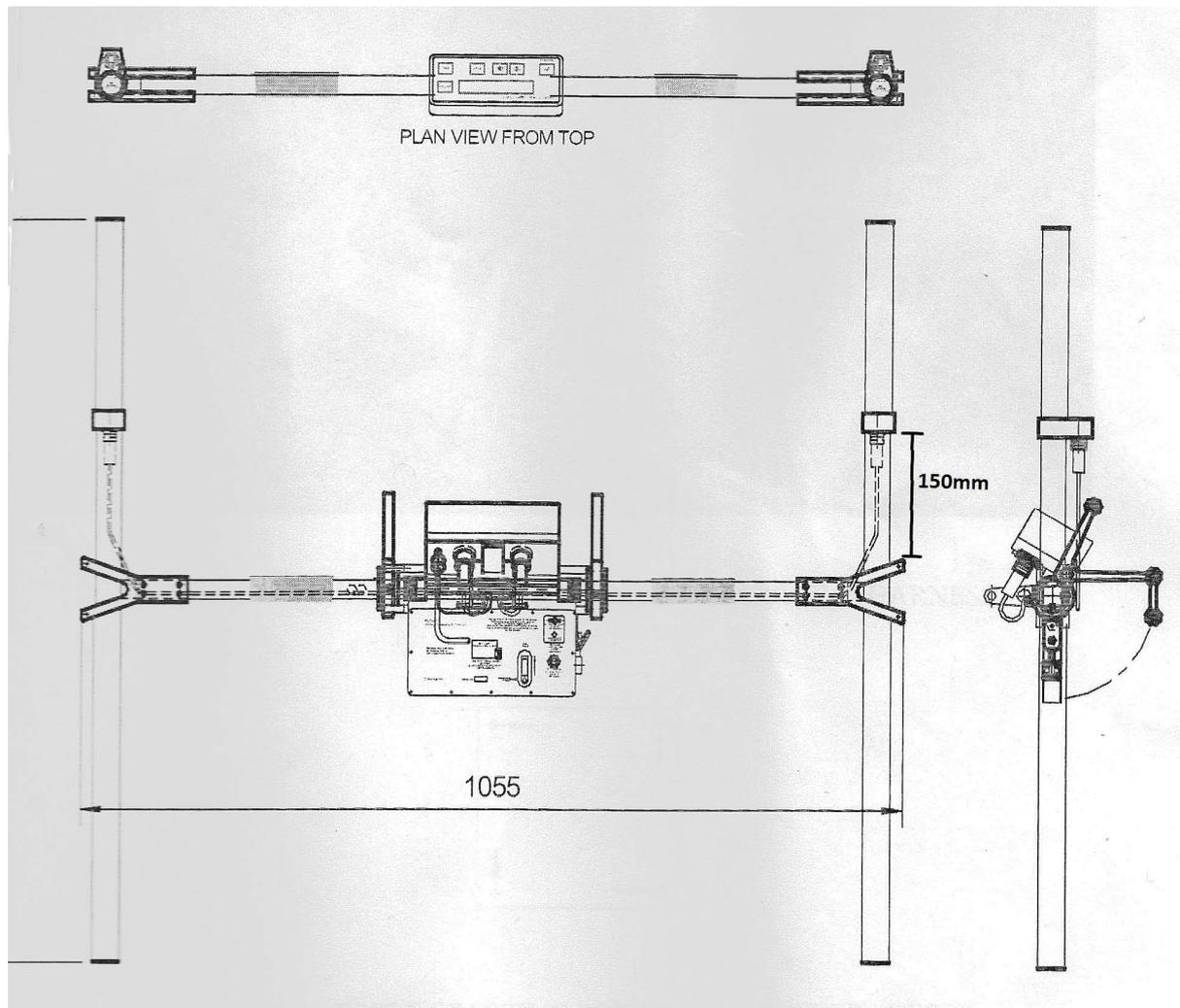
Figure 4.1 Bartington 601 Fluxgate gradiometer (Instrument instruction manual)
