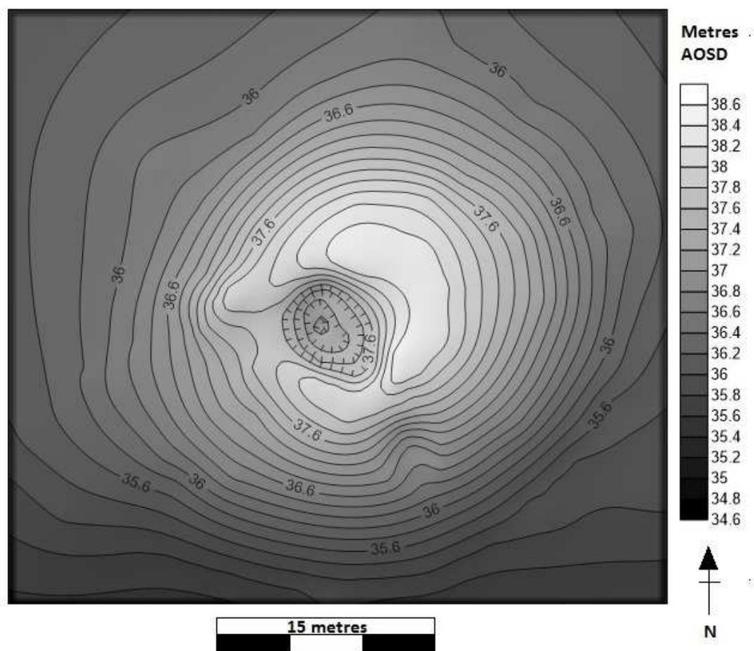
Figure 5.45 Topographic survey of Mound A viewed in plan from directly above
