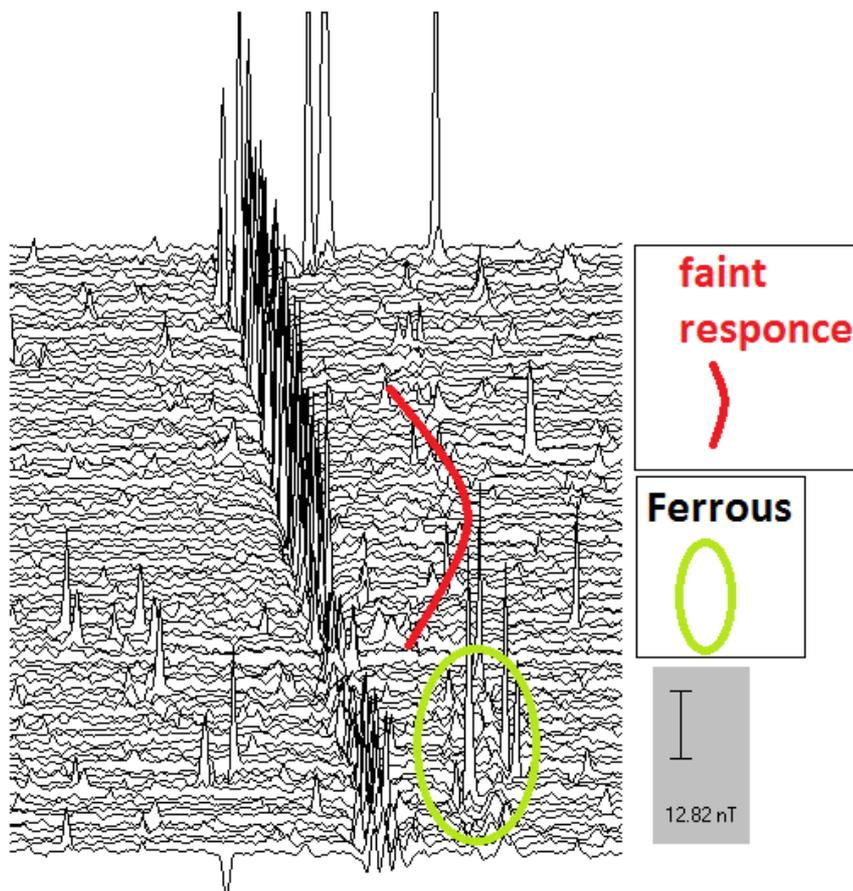
Figure 5.9 X-Y plot of Brockhall gradiometer survey with interpretation
