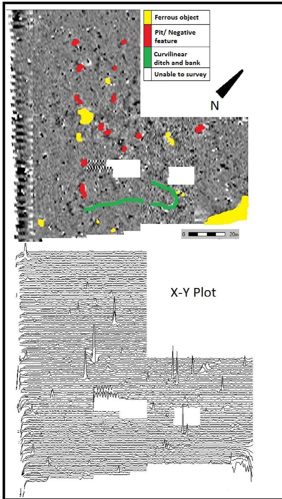
Figure 5.25 X-Y plot and interpretation of the features identified during the gradiometer survey of Area 2
